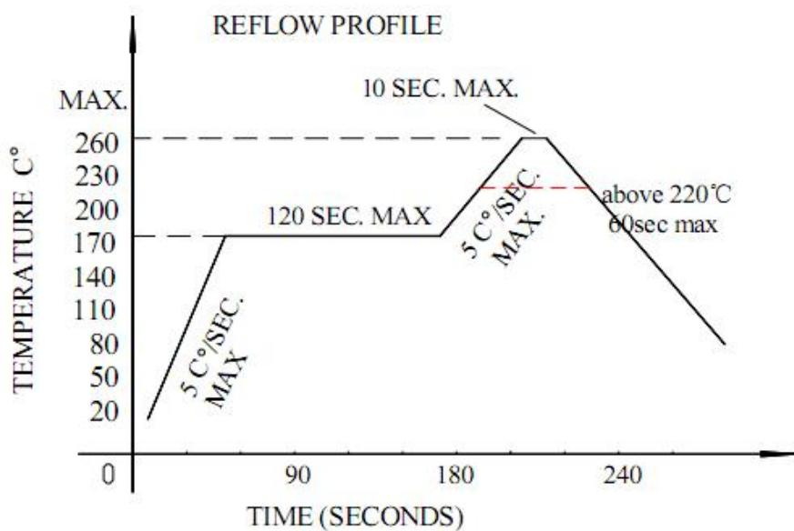
1. Reflow soldering should not be done more than two times
